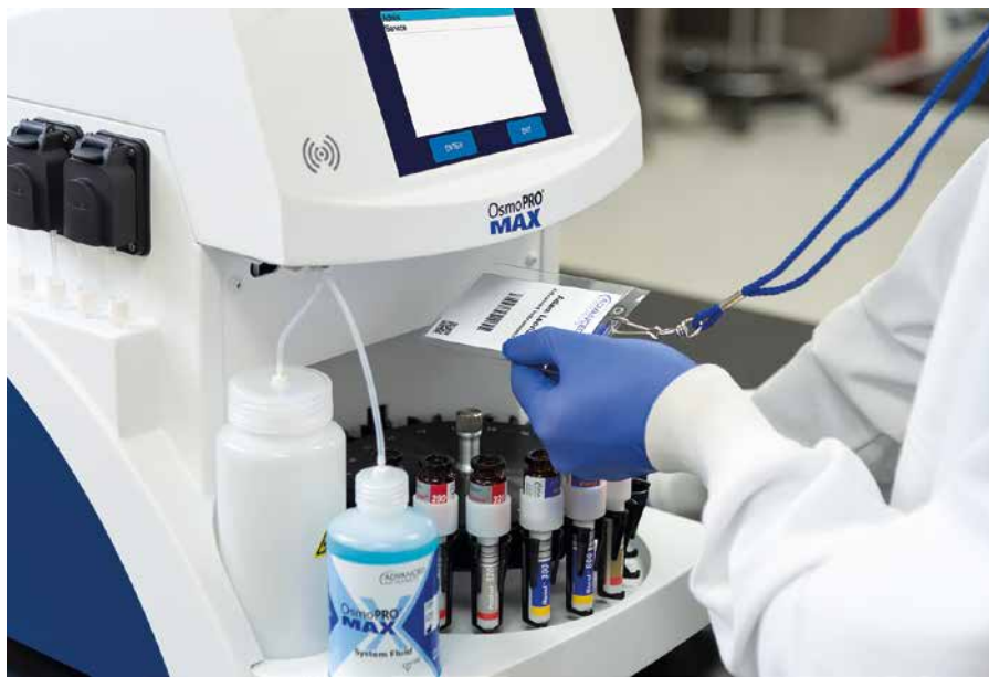
The OsmoPRO MAX's integrated barcode scanners trace users, minimise errors and simplify the testing process.
