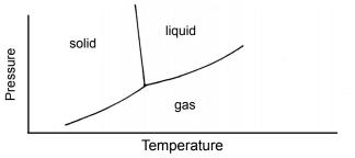
Figure 5: Phase Diagram for a Solvent
