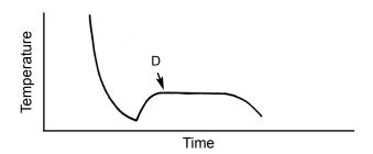
Figure 11: Solution Freezing Curve in a Cryoscope
