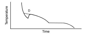
Figure 10: Solution Freezing Curve with Supercooling
