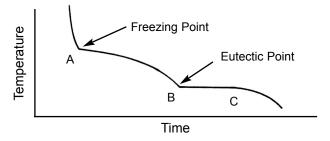
Figure 9: Solution Freezing Curve "Ideal"
