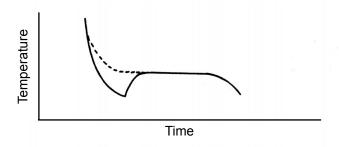
Figure 8: Solvent Freezing Curve with Supercooling
