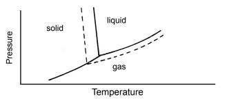
Figure 6: Phase Diagram with Addition of Solute
