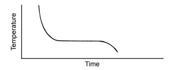
Figure 7: Solvent Freezing Curve "Ideal"
