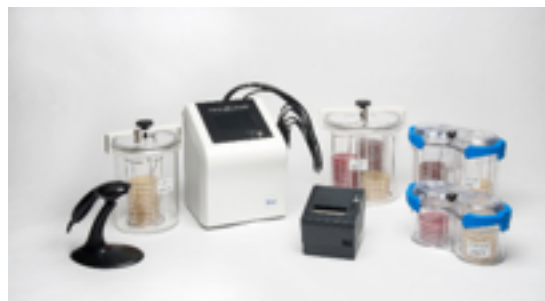
Figure 5.0: The Anoxomat III Jar System is pictured in the figure, equipped with four jar attachments. The instrument can be used with ergonomic (blue handle jars) in 12/24 plate format or the standard jars (white lids) in 12/26 plate format. Additionally, a hard copy of the data for each run can be printed by the thermal printer, pictured (or dot matrix printer, not pictured); alternatively data can be scanned and recorded digitally with the track and trace package and/or the bar code scanner (bottom left).
