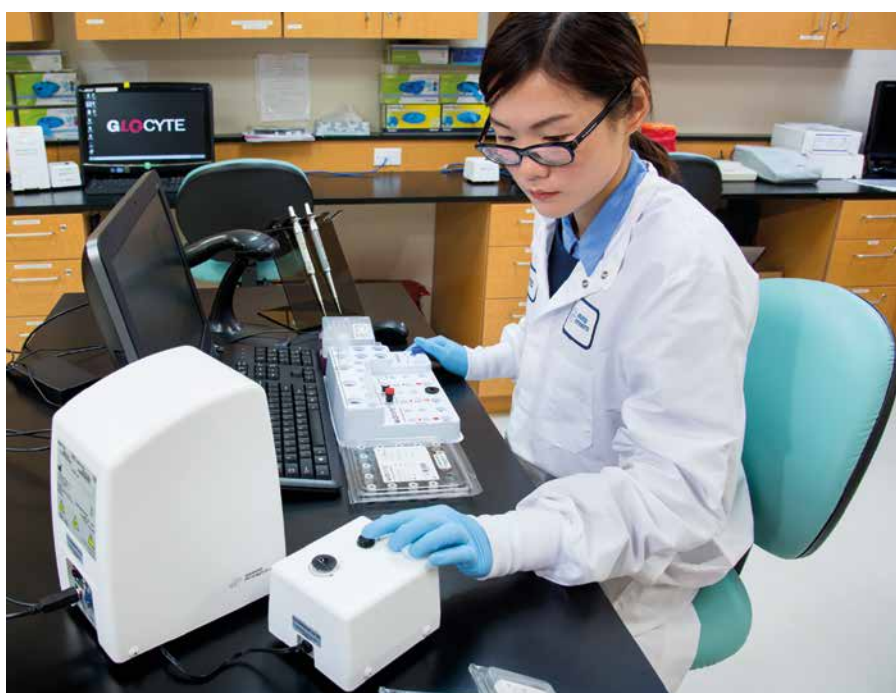
The GloCyte Automated Cell Counter System uses fluorescence microscopy and two reagents to enumerate total nucleated cells (TNCs) and red blood cells (RBCs) in under five minutes.
