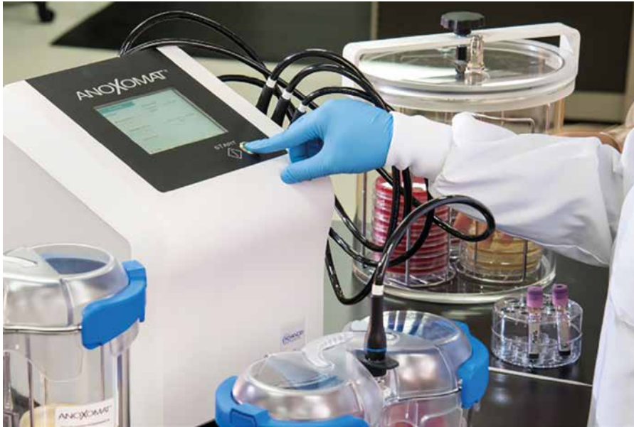
The Anoxomat anaerobic jar system is able to quickly create optimal conditions for the growth of anaerobic, microaerophilic, and capnophilic organisms.
